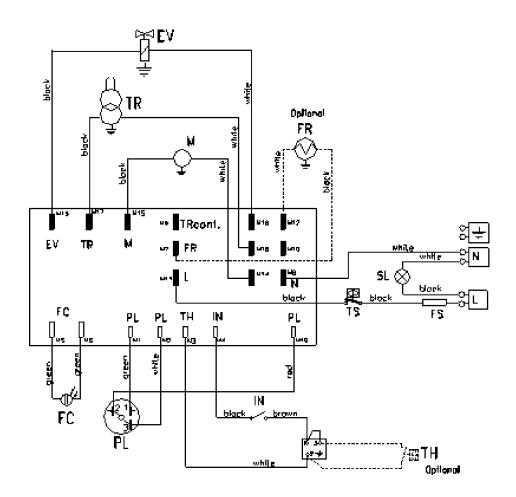
ΕV Fuel Solenoid Valve TR Ignition Transformer Motor Μ SL Warning Lamp TS Safety Thermostat FS Fuse FC Flame Sensor  $\mathsf{PL}$ Reset Button IN Switch Room Thermostat (Optional) Heated Filter (Optional) TH FR
